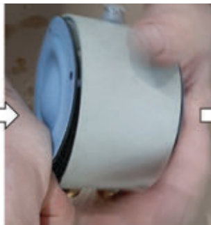
STEP 7: Unscrew the diaphragm from the body of the pump
