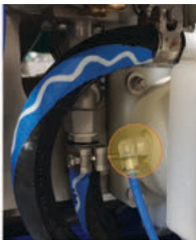
STEP 1: Unplug the compressed air supply hose
