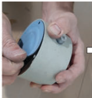
STEP 7: Unscrew the diaphragm from the body of the pump
