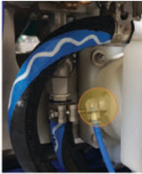
STEP 1: Unplug the compressed air supply hose
