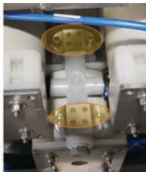
STEP 2: loosen the screws at the back of the pump
