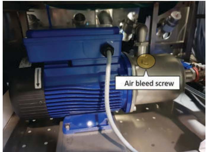
Fig. 23. Air bleeding the rotary pump
