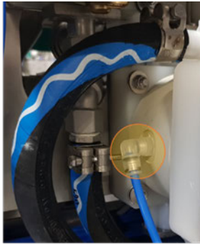
STEP 1: Unplug the compressed air supply hose
