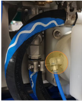
STEP 1: Unplug the compressed air supply hose
