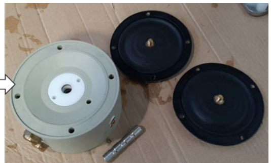
STEP 7: Pay attention not to scratch the pin when unscrewing it from the diaphragm.
