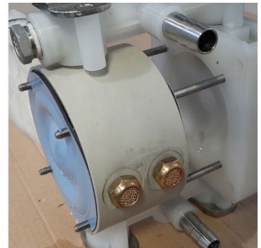
STEP 6: Gently remove the middle body of the pump mounted on the four pins
