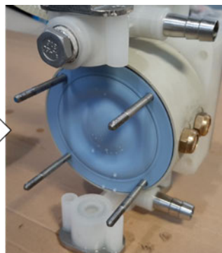
STEP 3: remove the screws at the front of the pump
