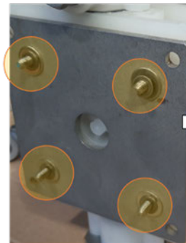
STEP 4: Unscrew four nuts fixed on pins, then remove the reinforcement plate.
