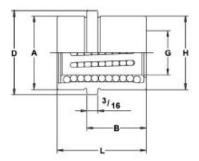
**GUIDE COLUMN** | BOLEXP guide column is made of steel 1.5732 with surface hardening, obtaining a hardness of 62-64 HRc, and a depth from 0.04 to 0.047 inches, leaving the shaft core soft so that it can absorb the bending it might be required to. In guide manufacturing, some features are considered to be essential, including the quality of steel, surface hardness and precision and quality of the finish.
