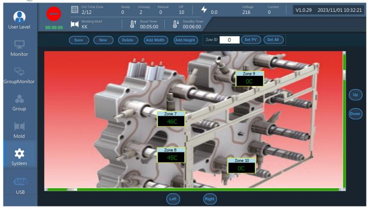
Rapid Understanding of Mold Structure and Temperature Distribution: Through visual representations, operators can instantly grasp the mold's structure and temperature distribution, which greatly facilitates rapid adjustments and optimization of mold performance.
