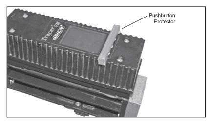
Tracer<sub>VM</sub> Interface and Sensor are calibrated as a matched pair. Separating the pair voids the calibration.
