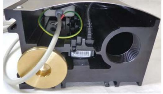
The manifolds can be mounted on machine platens or the mold with “roll-in” “T-nuts” which fit in Integrated extruded slots, which are located on two faces of the extrusion. The compact slim line design of the manifold enables it to be mounted in the smallest space possible next to the machine, on platens or on the mold, keeping the pipe runs to the absolute minimum.
