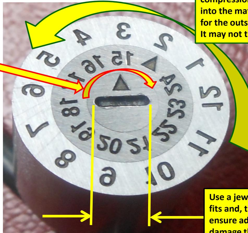
Use a jeweler's screwdriver that fits and, the tip fills the slot, to ensure adequate torque and not damage the edges of the slot (as shown above).
