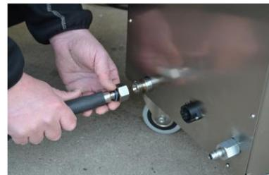
Plug the male electrical connector on the blast hose into the female socket on the front of the blaster by inserting the plug and securing by twisting clockwise.
