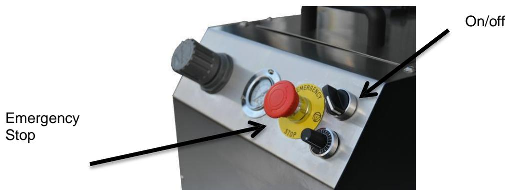
Turn the on/off switch to the right to turn on the machine and left to switch off.
