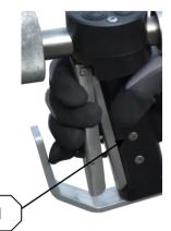
The blast gun has for safety been equipped with a safety pin (1) at the trigger. In order to activate blasting the lever most be pushed down, which in turn allows the trigger to be pressed.
