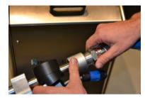
The blast hose has got two different threaded couplings. One will fit to the
